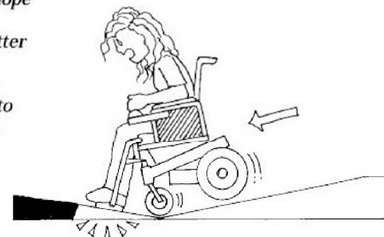
INCORRECT SIDEWALK RAMP
