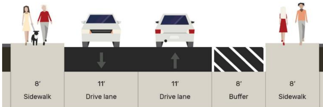
Figure 11: Short-Term Striping Alternative along Washington Street
