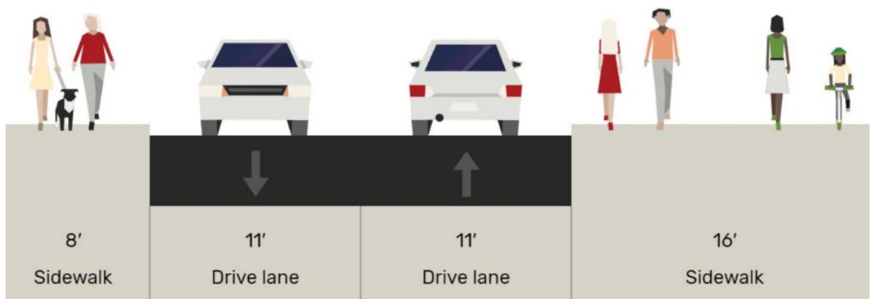
Figure 14: Long-Term Curb Extensions Alternative along Washington Street
