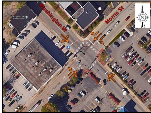
Figure 4: Washington Street and Morris Street Lane Configuration
