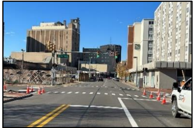
Photo 3: Inconspicuous Signal Heads at Washington Street and Leon Sullivan Way
