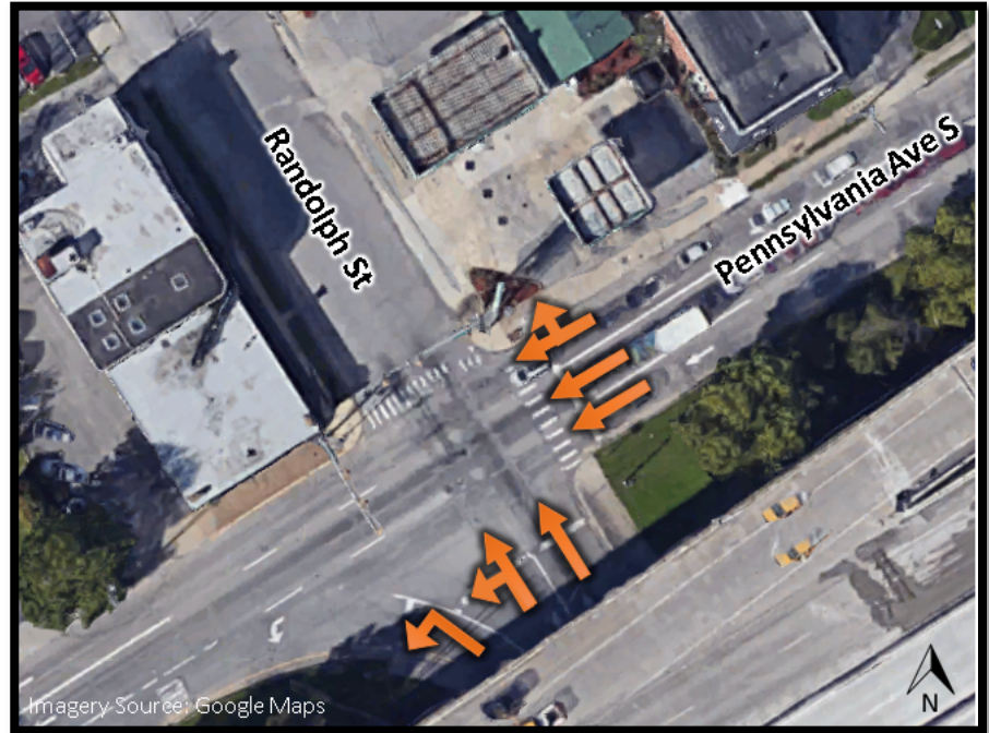
Figure 8: Pennsylvania Ave S and Randolph Street Configuration
