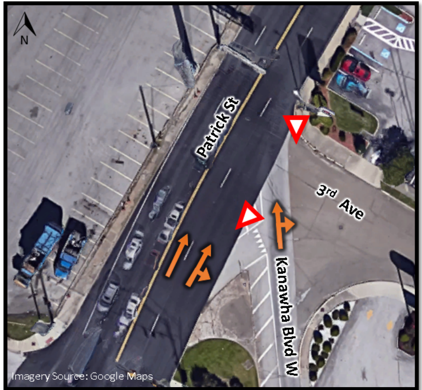
Figure 3: Patrick St and 3 rd Ave Lane Configuration
