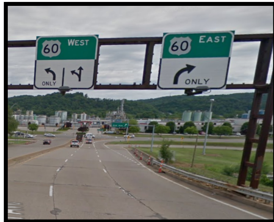
Photo 7: Overhead Lane Use Signs
