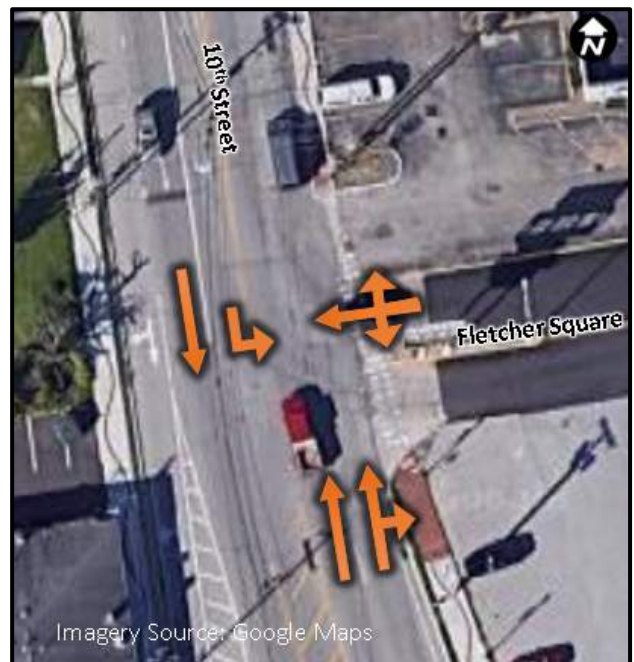
Figure 3: 10 th Street and Fletcher Square Lane Configuration
