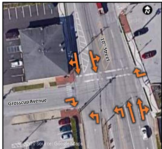
Figure 4: 10 th Street and Grosscup Avenue Lane Configuration
